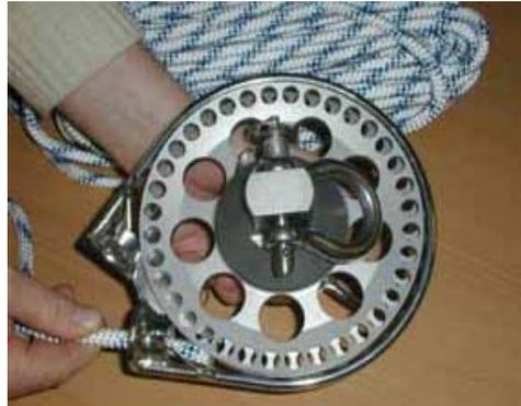
**The furling line has to be spliced and be careful on the Ø the splice to allow to pass through the furler.**
